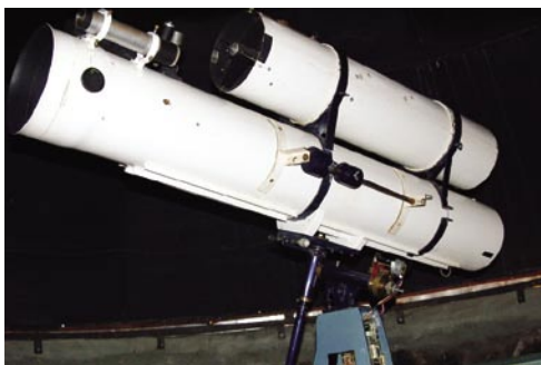
Figure 7. type reflector, diameter 28 cm, luminosity f8, eye-glass interchangeable
