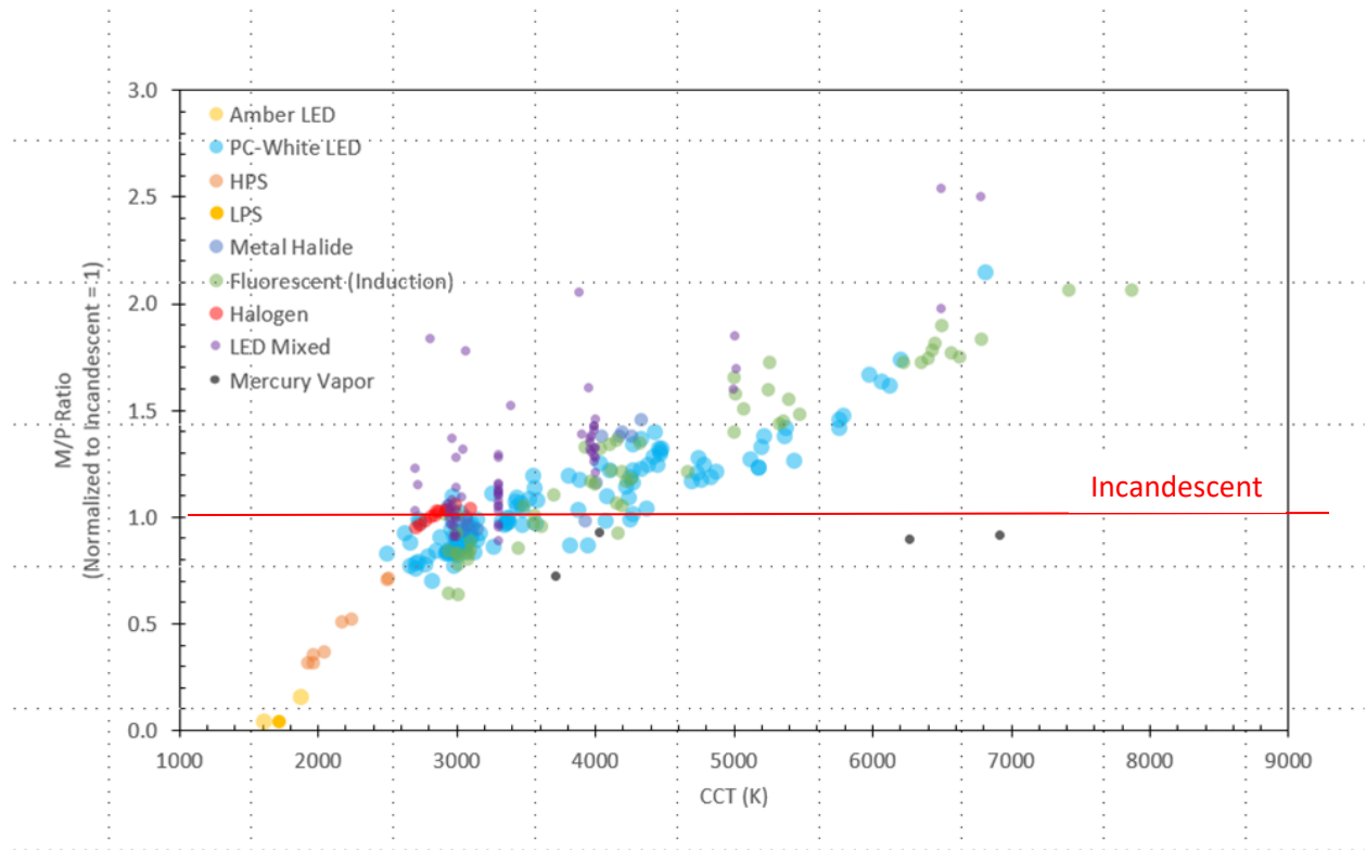
Figure 7. Calculated M/P ratio vs. CCT for a wide range of light sources, relative to incandescent.
